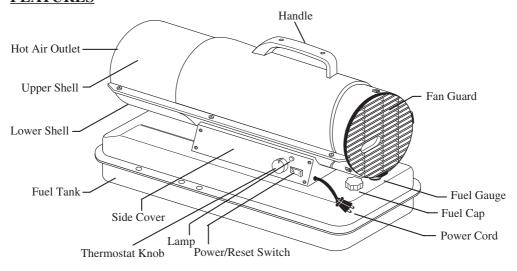
Figure 1. RMC-KFA45T / RMC-KFA65T MODELS
